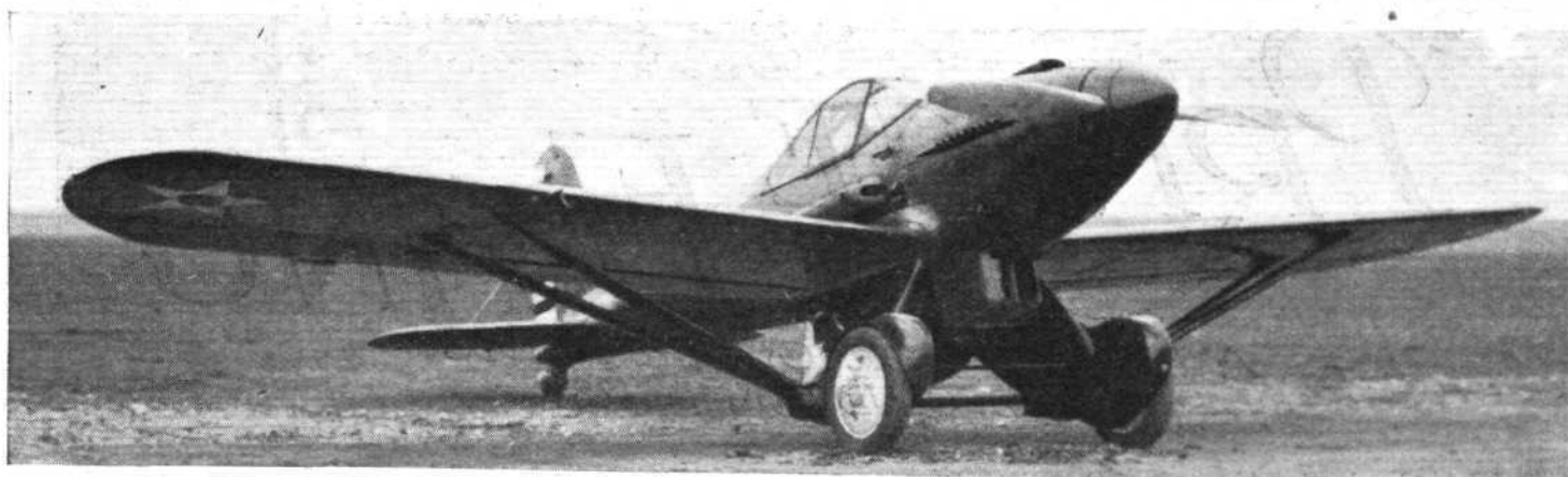
THE CURTISS "SWIFT": Note the enclosed cockpit. The engine is a "Conqueror."
