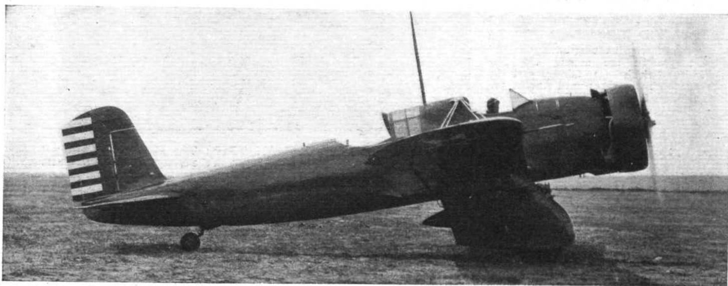
FOR GROUND STRAFING: The Detroit (or Lockheed) A-9 seen in the upper photograph has a Curtiss "Conqueror" engine, while the Curtiss A-12 in the lower picture has the Wright "Cyclone" radial air-cooled.
