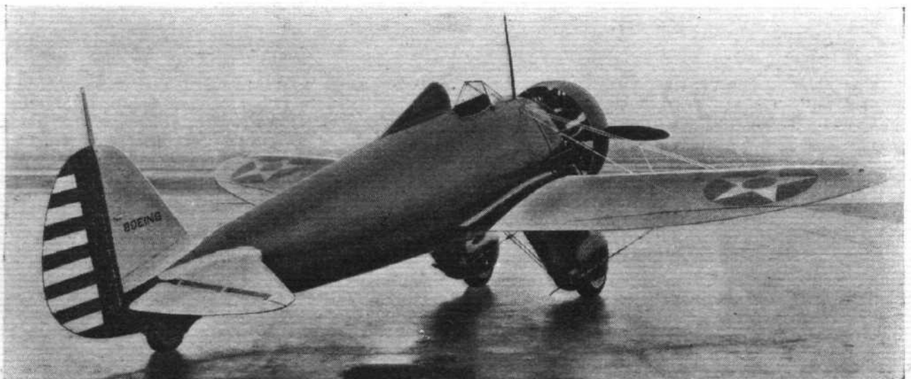
A PURSUIT TYPE : The Boeing P-26. The engine is a Pratt and Whitney "Wasp" of about 600 h.p.
