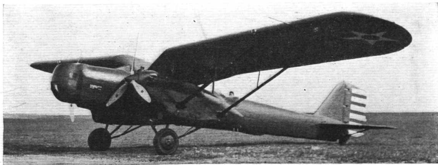
THE DOUGLAS VERSION: Like the Fokker o-27, the Douglas o-35 is an Army Observation type. It has the same type of engines, but is strutbraced and has the "gull's wing" formation.
