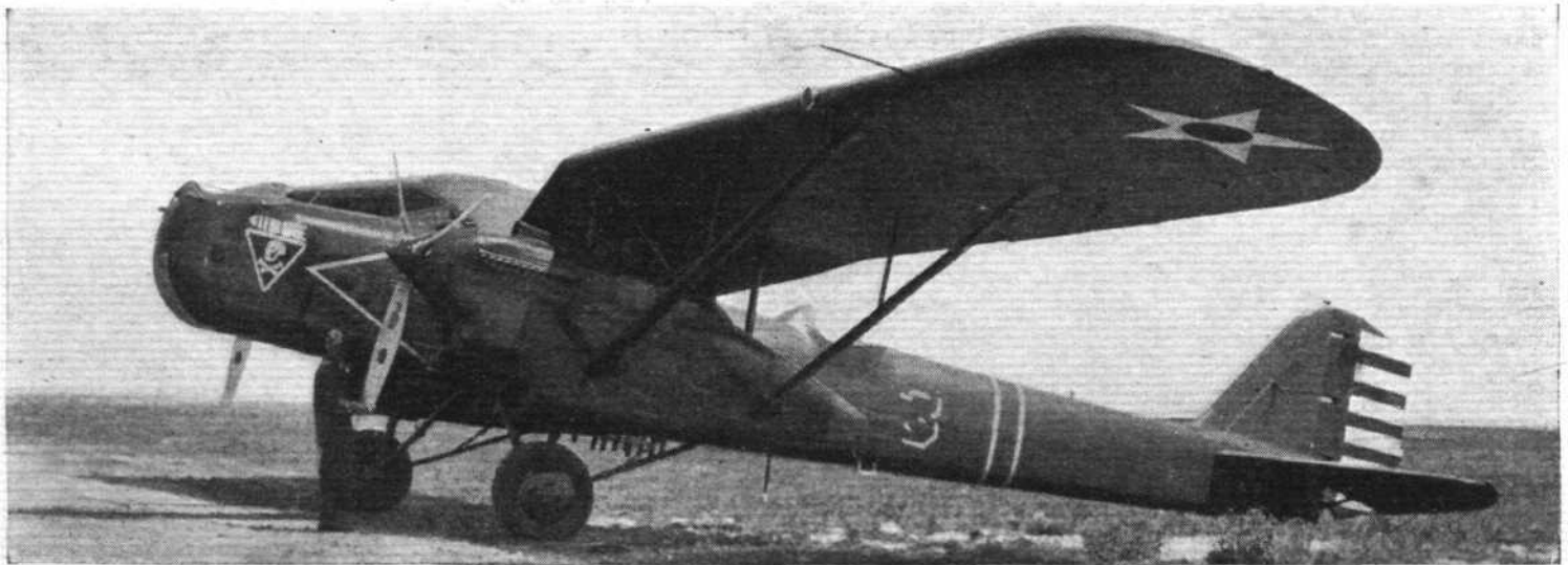
A BOMBARDMENT TYPE: The Douglas B-7 is powered by two Curtiss "Conqueror" engines of 650 h.p. each.
